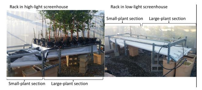
The design was specifically to allow randomization of plants growing in Proptek pots. The difficulty is to keep the leachates from the two recirculation treatments from mixing. The system has two reservoirs for the large-plant trails and two for the small-plant trials; in both cases, one for the recirculated treatment, the other for the non-recirculated treatment (see photos).
